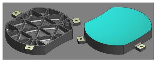
Figure 2. Mechanical design of the FLEX HRM Mirror.
