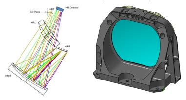
Figure 1. Optical layout of the FLORIS high-resolution spectrometer showing the HRM mirror (left) and view of the optomechanical assembly of the HRM mirror (right).
