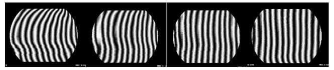
Figure 5. Evolution of the surface accuracy of the HR Mirror Breadboard during the IRP figuring and polishing runs.
