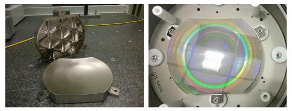
Figure 3. Two HRM mirror blanks after NiP coating (left) and one in the transportation container after final diamond machining (right).
