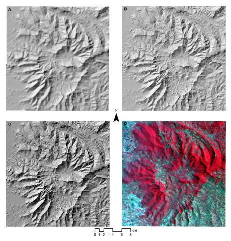
Figure 2. Hillshade of Digital Elevation Model used in this study, (a) SRTM, (b) AW3D, (c) DEMNAS, and (d) False-color composite of LAPAN-A3 data of the same area. Hillshade at the sun azimuth of 315° and the sun altitude of 45°.
