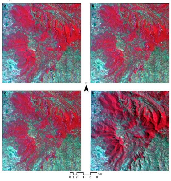
Figure 3. Visual comparison of topographically corrected LAPAN-A3 using Minnaert Correction using different DEM, (a) SRTM, (b) AW3D, (c) DEMNAS, and (d) Original LA3 image. All images are shown in the RGB composite of NIR-R-G.
