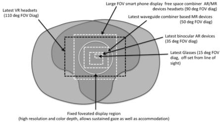
Figure 10: Typical FOVs for current state of the art Smart glasses, AR, MR and VR headsets, overlaid on the human binocular vision and the fixed foveated display region. One other way to describe the FOV experience is to overlap the amount of unobstructed see though FOV over the actual display FOV (see **Figure 1**). The fixed foveated region (scanned through eye movements) is shown in dotted lines.
