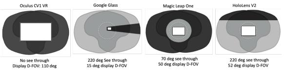
Figure 11: Display FOV and see through FOV for various VR, smart glasses and AR headsets.
