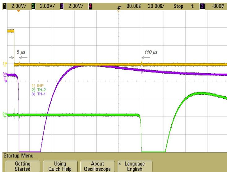
Figure 4. Measurement of delay time (yellow - imp. from a generator, equivalent to an impulse from an impact sensor, violet - activation of the TH-1 precursor detonation system, green - delayed activation of the TH-2 main charge system).
