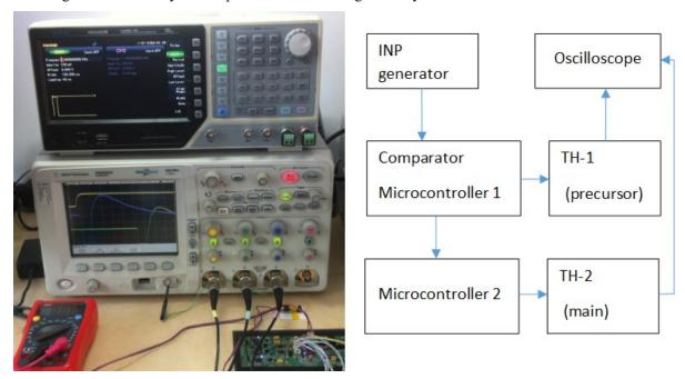
Figure 3. Laboratory test rig for programmable tandem detonator.
