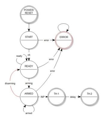
Figure 2. State machine algorithm of a programmable tandem detonator.
