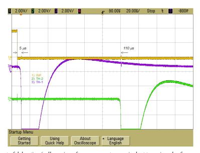
Figure 4. Measurement of delay time(yellow - imp. from a generator, equivalent to an impulse from an impact sensor, violet - activation of the TH-1 precursor detonation system, green - delayed activation of the TH-2 main charge system).
