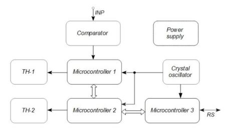
Figure 1. Block diagram of the programmable electronic tandem detonator.
