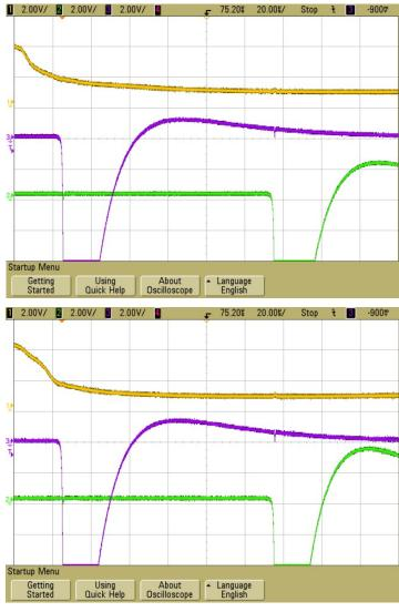
Figure 5. Measurement of delay time with resistance pressure sensor, 2 tests (yellow - imp. from a generator, equivalent to an impulse from an impact sensor, violet - activation of the TH-1 precursor detonation system, green - delayed activation of the TH-2 main charge system).
