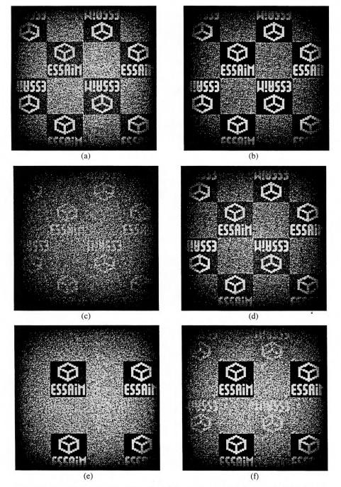
Fig. 7: Simulation of reconstructions provided by various implementations of DOE's: binary amplitude (a), 8-level amplitude only that is, at the moment, only possible in simulations (b), 8-level amplitude only displayed with a parasitic phase ranging from 0° to 360° (c), ), 8-level amplitude only displayed with a parasitic phase ranging from 0° to 83° (d), 8-level ideal 360° spiral (e), 8-level experimental spiral with (45°,-45°) configuration (f).
