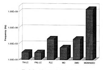
Fig. 2: Operating rate of various SLM's.
