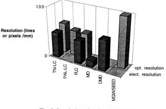
Fig. 3: Resolution of various SLM's.
