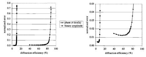
Fig. 4: Example of optimal characteristics curve (OCC) for the binary coding domain (from ref. <sup>43</sup>). The view on the right consists of a close-up of the view on the left.
