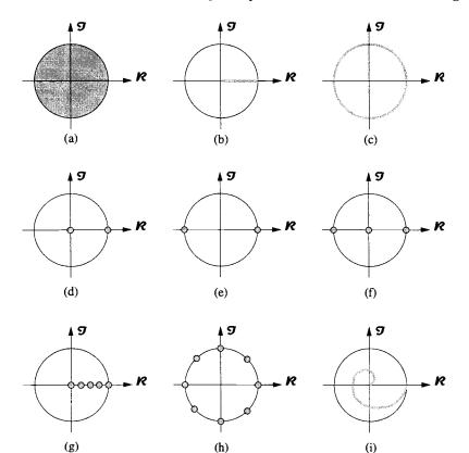
Fig. 1: Examples of coding domains: unity disk (a), pure amplitude (b), pure phase (c), amplitude only (d), pure binary phase (e), ternary phase (f), quantified amplitude only (g), quantified phase only (h), spiral (i)
