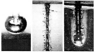
figure 8: Excimer laser-tissue interaction. Left: bubble during ablation in transparent tissue model, middle: collapsed channel with small fissures alongside, right: thermal effects along channel wall during tissue penetration with fiber
