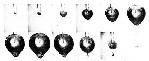
figure 2: Sequence of an expanding and imploding vapor bubble induced by a holmium laser pulse in water. The frames are 50  $\mu s$  apart totally covering  $\sim 600~\mu s$ .
