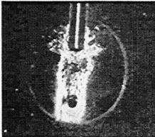
figure 5: Left: shock waves induced by cavitation bubbles, notice the kernel at the center of each spherical wave. Right: shock wave induced at the implosion of a holmium vapor bubble.
