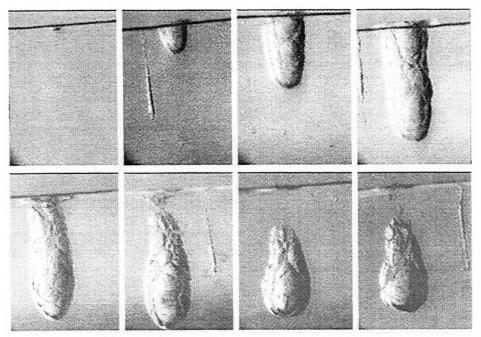
figure 3: High speed image sequence of a deep channel formed during tissue irradiation with a 300 µs focussed erbium laser beam.
