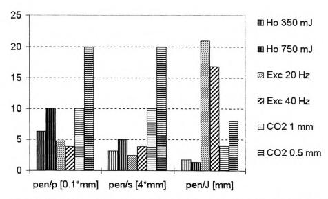
figure 9: Comparison of the penetration efficiency of laser systems typically used for TMLR. Laser settings for Holmium: 350 mJ and 750 mJ at 3 Hz, 1 mm fiber tip. Laser settings for Excimer: 30 mJ at 20 and 40 Hz, 1 mm fiber tip. Laser settings for CO<sub>2</sub>: 350 mJ focussed to 0.5 and 1.0 mm spot at 3 Hz.
