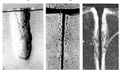
figure 6:  $CO_2$  laser-tissue interaction. left: expanded channel during ablation, middle: collapsed channel with small cracks alongside, right: thermal effects along channel wall directly after the laser pulse.
