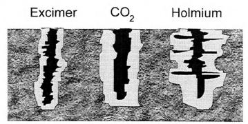
figure 10: general features of the channels created with three laser modalities showing the extent of thermal damage and mechanical fissures in the wall.
