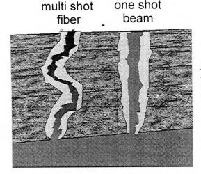
figure 11: schematic comparison between channel created with fiber delivery and channel created in one shot by a focussed beam.
