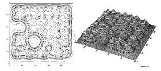
Fig. 4 - Measured relative SAR distribution 1 cm deep in muscle phantom from a 16 element array of 4 cm square DCC apertures spaced 1.5 cm apart, radiating through a 12 mm thick water bolus. Two apertures are off to demonstrate the resolution of power control of the antenna array. The two bold lines are 25% and 50% of SAR<sub>max</sub>.
