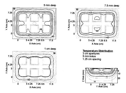
Fig. 6 - Temperature distribution predicted 5, 7.5 and 10 mm deep in muscle and central y-z cross section under 6 element array of 3 cm square DCC apertures coupled with 5 mm water bolus. Blood perfusion is assumed to be  $2 \text{ kg/m}^3$ s, water bolus temperature is 42°C and highest temperature point in tissue is 45°C. Note the 42°C contour in bold extends to the array perimeter down to 1 cm depth in muscle.
