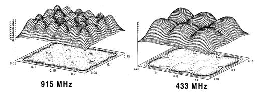
Fig. 5 - FDTD calculated SAR pattern 1 cm deep in muscle phantom under 6 element array of 4 cm square DCC apertures spaced 1.5 cm apart and coupled with 6.25 mm thick water bolus and driven at 915 or 433 MHz. Note that the bold contour, which represents 50% of SAR<sub>max</sub> in the 1 cm deep plane, extends to the array perimeter demarcated by the dashed aperture outlines.
