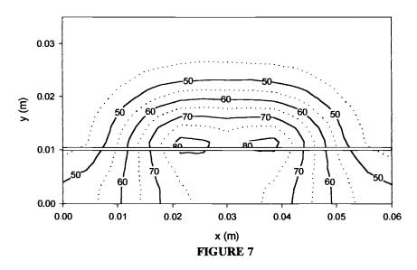
The figure shows isotherms for three electrodes mounted on an air-filled, silastic balloon in uterine tissue activated with RF monopolar energy. The electrodes are multiplexed and ground is the top surface. The results are for the end of treatment at 4 minutes.
