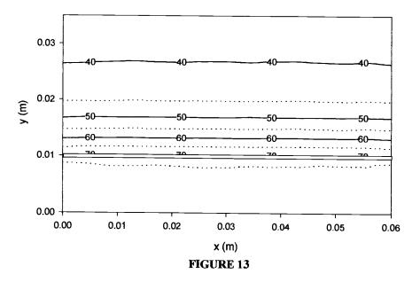
The figure shows the results of a temperature distribution calculated for a fluid-filled balloon at 15 minutes, with the assumption that the fluid circulates and is controlled at 76°C.
