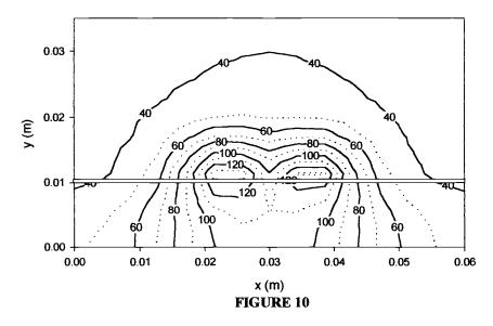
The figure shows isotherms for three electrodes mounted on an air-filled, silastic balloon in uterine tissue. The electrodes are operated in a bipolar fashion with a voltage applied to either side electrode relative to the center electrode. The results are for the end of heatup at 1 minute.
