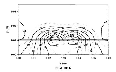
The figure shows isotherms for three electrodes mounted on an air-filled, silastic balloon in uterine tissue activated with RF monopolar energy. The electrodes are multiplexed and ground is the top surface. The results are for the end of heatup at 1 minute.
