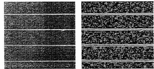
Figure 2. A broken lose thread on a fabric of the type showed in figure 1. Edge detection may be successful if previous smoothing is performed.
