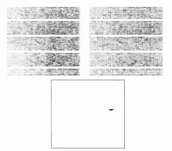
Figure 4. Subtracting the two images after white dilatation gives the identification of the out of place thread tip. Blob analyzes allows evaluation of its size (3 mm long, 1 mm thick).
