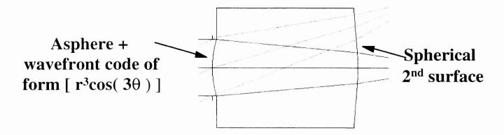
Fig. 11. A single-element hybrid imaging system with wavefront coding to extend the depth of focus and signal processing to restore the OTF.
