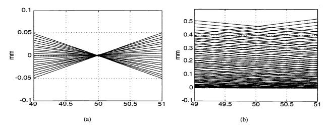
Fig. 2. Ray traces for (a) conventional lens, and (b) effect of the phase plate on the ray trace. Note the change in the vertical scale.
