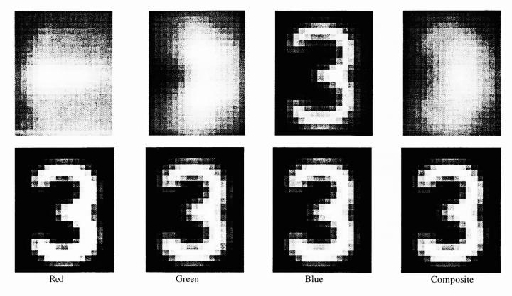
Fig. 10. Images of the numeral 3, showing the effects of axial chromatic aberration with a conventional imaging system (top), and a hybrid digital/optical system (bottom).
