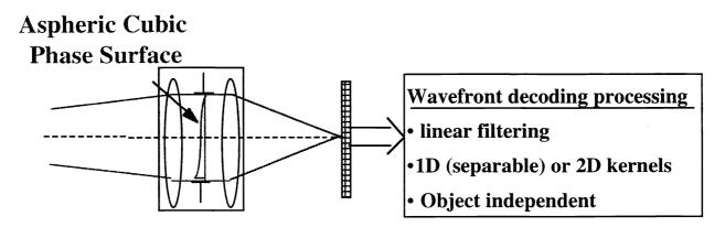
Fig. 1. Schematic of hybrid optical/digital imaging system. The intermediate image is acquired by the detector array, and the final image is produced by signal processing.
