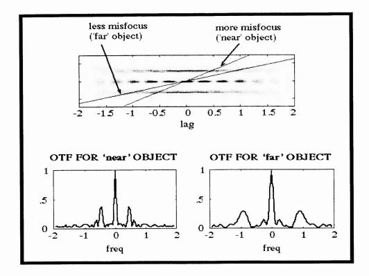
Fig. 5. The effect of the misfocus, or range of the object on the OTF for a hybrid digital-optical system that was designed to "image" range.
