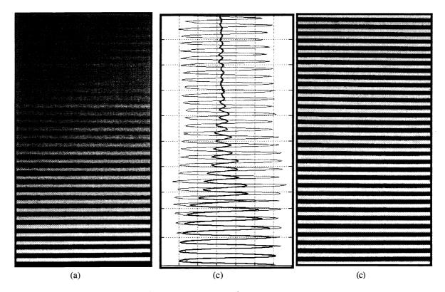
Fig. 4. Images of a bar pattern that has been inclined by  $60^{\circ}$ . The camera was focused on the bottom of the bar pattern. The left image was formed by a conventional imaging system. The right image was formed by a hybrid imaging system to extend the depth of field. The traces in (b) are through the center of the two images of a bar. Note the contrast reversal of the image formed with a conventional system.
