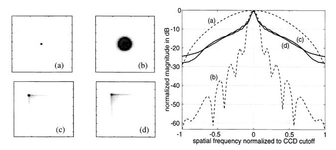
Fig. 3. Measured values of the PSFs and the MTFs for a conventional imaging system (a and b) and for the optical portion of the hybrid system ((c and d) of Fig. 1. The corresponding MTFs are shown to the right.
