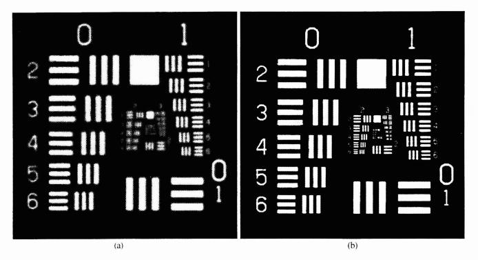
Fig. 8. A color image of an Air Force resolution test chart showing the images taken with (a) conventional imaging system, and (b) hybrid digital/optical imaging system.
