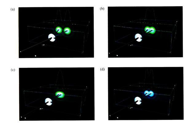
Fig.3 Rayleigh Resolution Module. (a) wavelength = 550 nm, diameter = 3.355 nm, angle =  $4.0 \times 10^4$  rads. The images are resolved. (b) wavelength = 550 nm, diameter = 3.355 nm, angle =  $2.0 \times 10^4$  rads. The images are barely resolved. (c) wavelength = 550 nm, diameter = 3.355 nm, angle =  $1.0 \times 10^4$  rads. The images are not resolved. (d) wavelength = 450 nm, diameter = 3.355 nm, angle =  $2.0 \times 10^4$  rads. The images are resolved.
