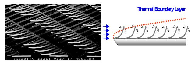
Figure. 7a. Bulk micromachined microfin array.
