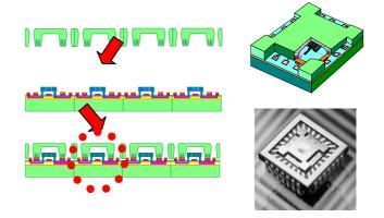
Figure 2b. Wafer-level vacuum packaged micro gyroscope
