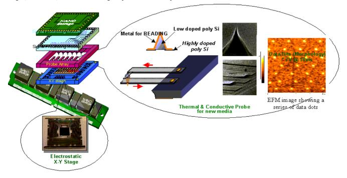
Figure 5. Next generation mobile/micro storage system.
