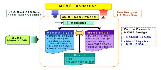
Figure 10. Concurrent Engineering CAD System for MEMS
