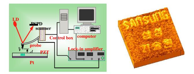
Figure 4. Use of electrostatic force microscope in writing high density data on thin PZT film.
