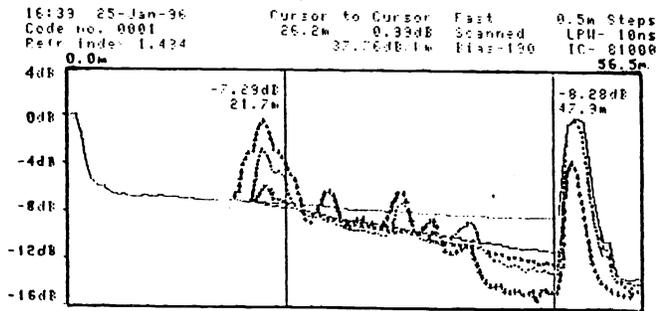
Figure 10a. Optical time domain reflectometer (OTDR) traces showing the development of non-uniform loss (slope of curve) related to core damage from the action of HF.
