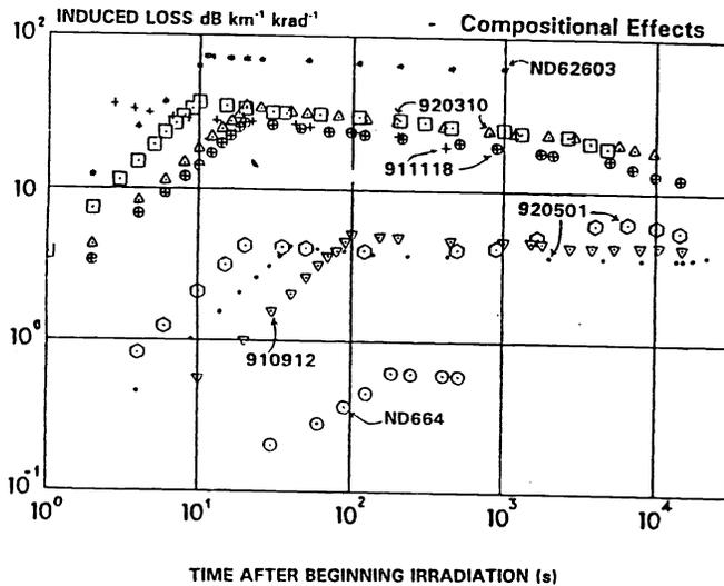
Figure 8. Losses during irradiation and recovery for a selection of Er doped fibres from a variety of sources and having different compositions. The same dose rate was used for all. In order to compare them the results have been scaled so that the recoveries (which tend to the corresponding RIRs at longer times) can be expressed in dB/km/krad..
