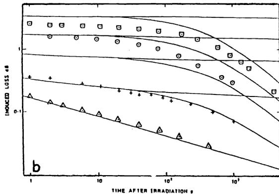
Figure 5a. Curves derived from the inset expression used to describe the RIR for undoped core fibres. Those shown are for  $A = 10$  (at 1s),  $D = 0.00133$  (light level 100nW), and for  $B$  from 0 to 400. Results (o) are for an all silica fibre at 100nW and 30 $\mu W$ ; for an HCS fibre (x) for thermal annealing and two light levels; the remainder (+) for a hardened PCS.
