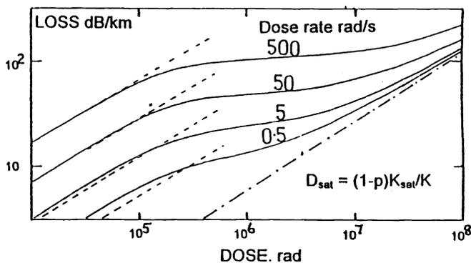
Figure 3. Losses in a Ge fibre (1300nm, 23°C) during constant rate, R , exposure to higher doses ( R = 0.5, 5, 50, 500 rad/s up from the lowest ). Dotted lines show extrapolations of the low dose, high rate, power law limit; dot/dash is the long term, low dose rate limit, assumed not to recover.
