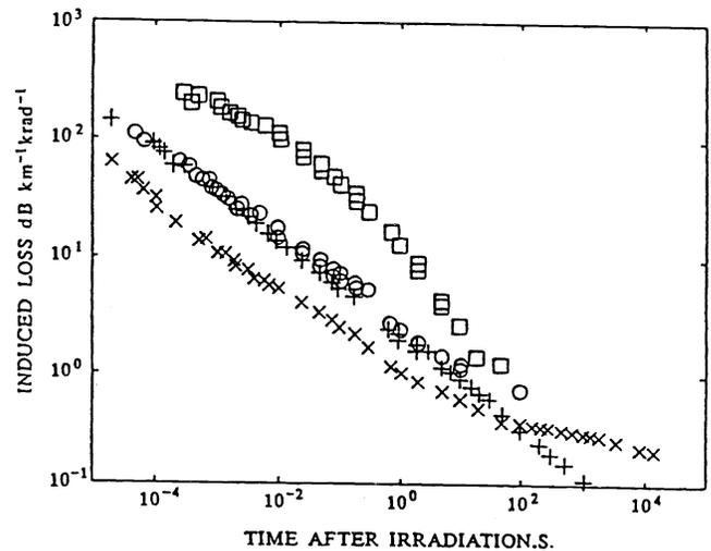
Figure 9. Recovery after pulsed irradiation for (+) Corning MM, (o) Philips MM, (x) Philips SM, and (□) 3M PMF, all at 23°C and for 1300nm, showing the greater sensitivity of the PM fibre, in this case at short times.
