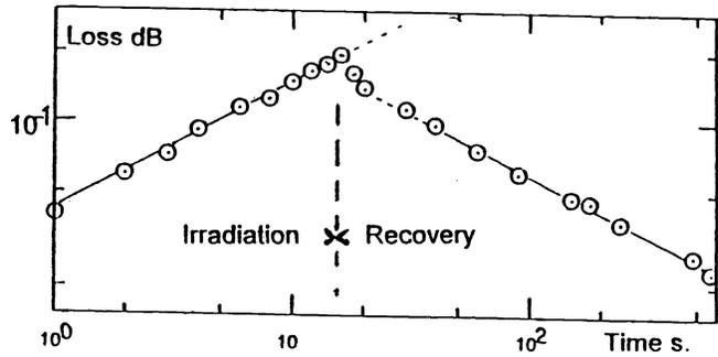
Figure 7. Loss during exposure at 100 rad/s, and subsequent recovery, for a 2m long, multicore fibre of Ce doped glass. It closely follows power law behaviour with an RIR  $\propto t^{-0.5}$ .
