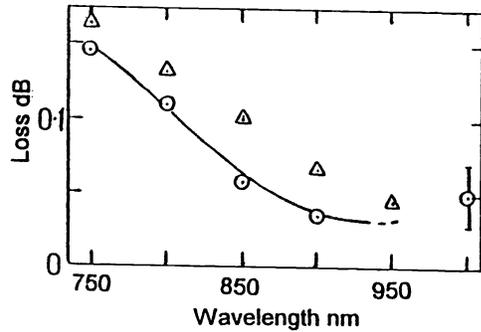
Figure 6. Losses after 150rad at 110 rad/s in 2m multicore fibres a)  $\Delta$  - lead glass, b)  $\circ$  - Ce doped glass. The line is to guide the eye. The lead glass experimental figures have been reduced by a factor of 25 before plotting. Thus, in this wavelength region, Ce doping can reduce losses by up to a factor of 50.
