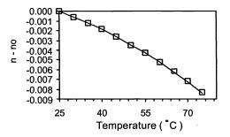
Figure 5. The experimental values of the index of refraction of water  $(\Box)$  as a function of temperature compared with the values calculated from references [3] and [4] (solid line).
