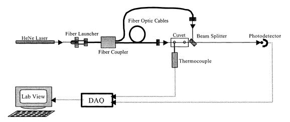
Figure 2. The fiber optic version of the Mach-Zehnder interferometer used as a refractometer.
