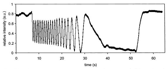
Figure 6. Signal from the photodetector as observed when air is let into the evacuated cell. The maxima and minima represent the variation from bright to dark fringe respectively. Going from one minimum to the next minimum via a maximum or one maximum to the next maximum via a minimum corresponds to a single fringe shift.
