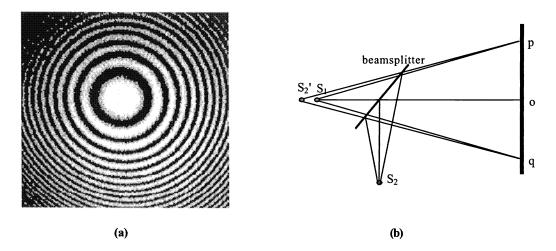
Figure 3: a)The 'bulls-eye' type of interference pattern. b) optical ray tracing of the interferometric set up
