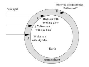
Figure 1. Relation of optical path length with the color of sky and sun.
