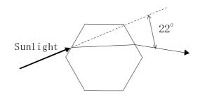
Figure 3. Schematic diagram of optical path for halo in crystallization of ice.
