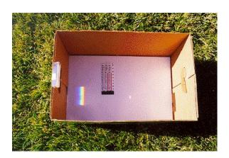
described by Sadler<sup>1</sup> (1991). When oriented properly, this setup projects a brilliant spectrum to the left and right of the center of the projected light.
