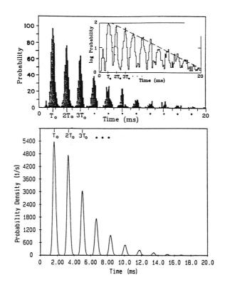
Figure 4. Upper panel: Interspike interval histograms (ISIH) of responses of auditory neuron subjected to weak stimulus with period 1.66 ms from reference.<sup>25</sup> Inset: data plotted on semi logarithmic scale. Lower panel: ISIH from an experiment with an electronic Schmitt trigger from reference.<sup>26</sup> In both cases the peaks are located at integer multiples of the stimulus period.
