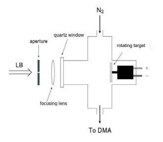
Figure 1. Schematic view of the experimental arrangement for nanoparticle generation by laser ablation. LB and DMA denote laser beam and differential mobility analyzer, respectively.
