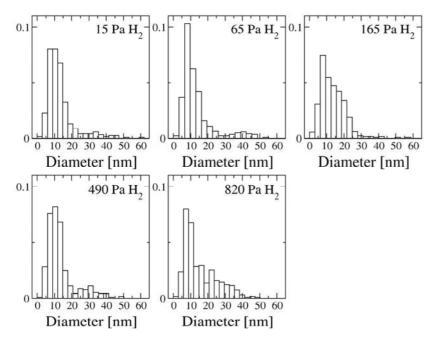
Figure 10. Normalized size-distribution histograms for five different H<sub>2</sub> partial pressures. Diameters of 400 particles were measured for each  $p_{H2}$  from TEM BF micrographs. WF<sub>6</sub> partial pressure 30 Pa with a total pressure of 2000 Pa.
