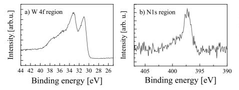
Figure 4. XPS spectra from polydisperse particles generated by ArF excimer laser ablation of W in  $N_2$  atmosphere. a) W 4f and b) N 1s regions, respectively.
