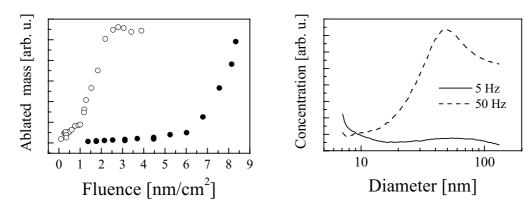
Figure 7. Ablated mass (integrated over the size spectra) versus laser fluence for WN<sub>0.3</sub> (solid points) and CN<sub>x</sub> nanoparticles (x ~ 0,1 open circles). The laser repetition rate was 2 Hz, spot diameters were 210 and 500  $\mu$ m for W and C ablation, respectively.
