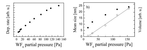
Figure 13. a) Rate of deposition of tungsten from XRF measurements, and b) mean size (diameter, solid points from Fig. 12), dependence on  $WF_6$  partial pressure. The open circles denote the mean volume of the particles derived from the mean size. H<sub>2</sub> partial pressure 165 Pa at a total pressure of 20 mbar. The solid line in Fig. b represents the best linear fit.
