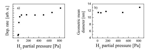
Figure 11. a) Tungsten deposition rate and b) geometric mean diameter of W nanoparticles as a function of  $H_2$  partial pressure, respectively. The deposition rate was measured by XRF, the mean diameter was determined by TEM measurements, see the histograms in Fig.10.
