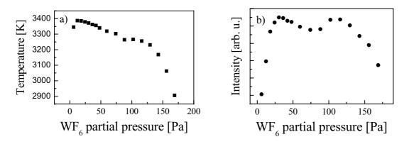
Figure 15. a) Temperature and b) intensity of the blackbody radiation as a function of  $WF_6$  partial pressure. Gate pulse 1  $\mu$ s, delay time 500 ns, H<sub>2</sub> partial pressure 165 Pa with a total pressure of 2000 Pa. Laser fluence 120 mJ/cm<sup>2</sup> and repetition rate 50 Hz.
