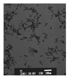
Figure 12. Left: Normalized size-distribution histograms for five different WF<sub>6</sub> partial pressures. Diameters of 400 particles were measured for each  $p_{WF6}$  from TEM BF micrographs. Right: TEM picture of agglomerated particles at 115 Pa WF<sub>6</sub> partial pressure. H<sub>2</sub> partial pressure 165 Pa with a total pressure of 20 mbar.
