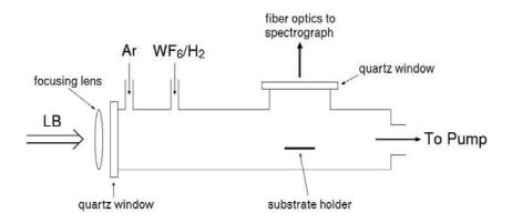
Figure 2. Experimental arrangement for laser-assisted deposition of tungsten nanoparticles. LB stands for laser beam.
