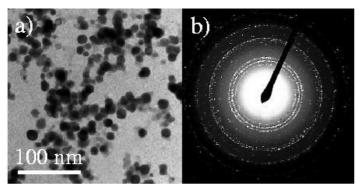
Figure 9. a) TEM image and b) electron diffraction pattern of LCVD deposited tungsten particles. Laser fluence  $120 \text{ mJ/cm}^2$ , 165 Pa H<sub>2</sub> and 115 Pa WF<sub>6</sub> partial pressures, total pressure 20 mbar.
