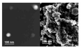
Figure 3. SEM micrographs from size-selected (40 nm in diameter) particles produced at  $\sim 8 \text{ J/cm}^2$  laser fluence at different deposition times. Left 5 minutes and right 45 minutes, respectively.
