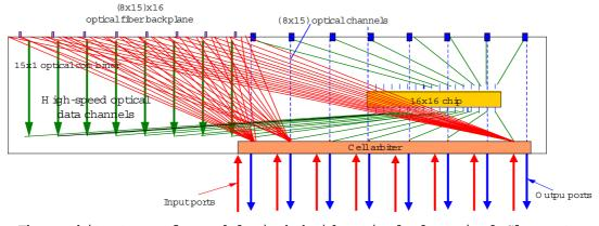
Fig.4. The architecture of a module in hybrid optical electrical Clos network for 128 hosts
