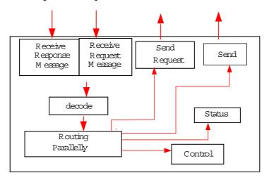
Fig.7 The block diagram of the InterRCU
