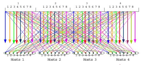
Fig.2, The passive optical fiber backplane for Cluster of 32-hosts
