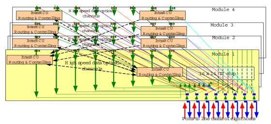
Fig.5. signaling control system of hybrid optical electrical Clos switch network The format of the signaling message is defined as follows:
