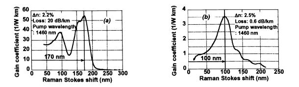
Figure 15 Raman gain coefficient spectra (a) Tellurite-based fiber (b) Silica-based fiber
