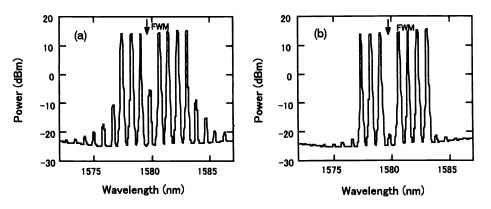
Figure 13 Output spectrum EDTFA : (a) sample A and (b) sample D
