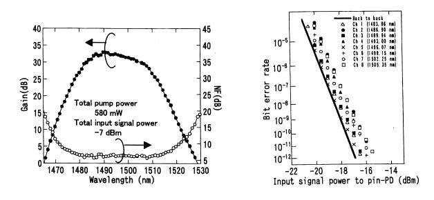
Figure 5 Gain and noise spectra of GS-TDFA
