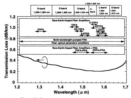
Figure 17 Gain spectra of various optical fiber amplifiers
