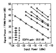
Figure 14 Power ratio between output signal and FWM
