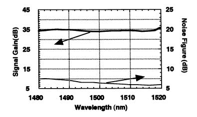
Figure 7 Gain and noise figure spectra of extended GS-TDFA
