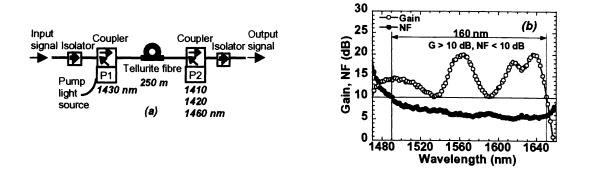
Figure 16 Multi-wavelength pumped tellurite-based FRA (a) Configuration (b) Small signal gain and noise figure spectra
