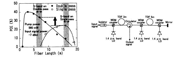
Figure 3 PCE for GS-TDFA dependence on fiber length
