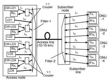
Fig.1 Schematic diagram of the WDM-PON system.
