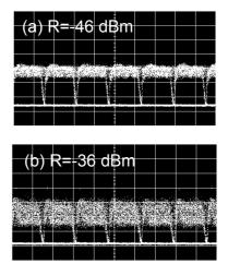
Fig. 4 Upstream signal eye diagrams for background reflections of (a) -46 dBm and (b) -36dBm.
