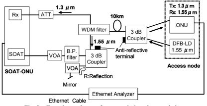
Fig. 2 Experimental setup for transmission characteristics.
