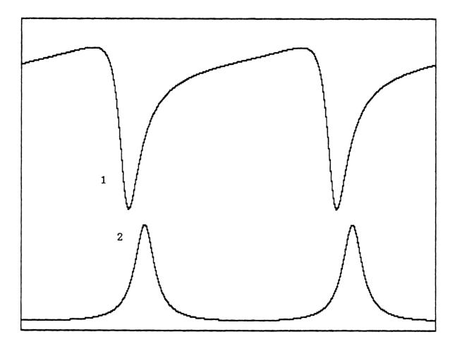
Fig.6. Computer simulated Fabry-Perot reflection (1) and transmission (2) spectra. Absorbtion coefficient a=0.13, R1 and R2 phase difference f=0.6.
