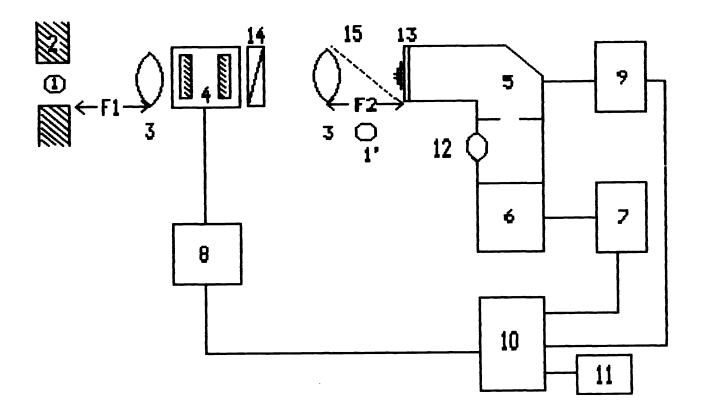
Fig.2. Spectral installation with Fabry-Perot etalon.
