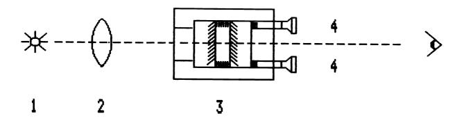
Fig.1. Set up for Fabry-Perot etalon adjustment. 1-mercury gas discharge lamp, 2-lense, 3-Fabry-Perot etalon, 4-screws and springs. Looking through Fabry-Perot etalon the student sees violet, green and yellow fringes. The center of the fringes always coincides with the image of his pupil.
