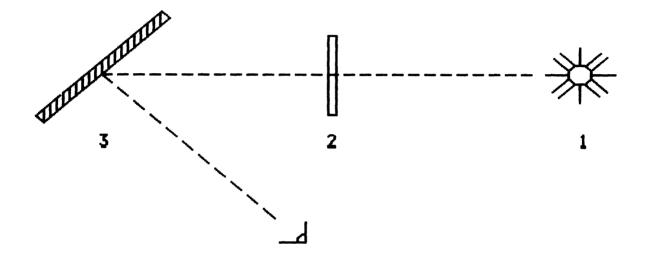
Fig.4. Simple demonstration set up. 1 - filament lamp, 2 - thin Fabry-Perot etalon, 3 - grating.
