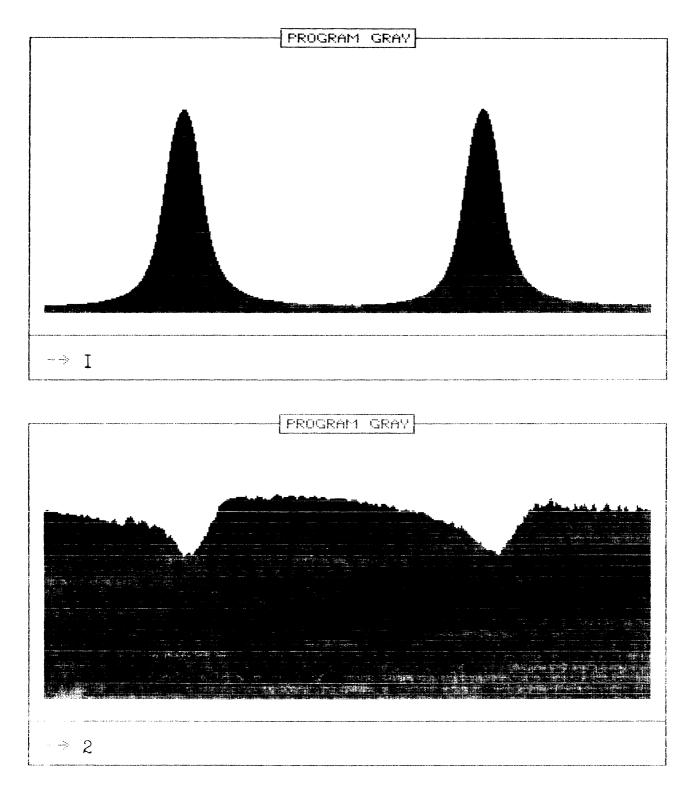
Fig.5. Fabry-Perot transmission (1) and reflection (2) spectra.
