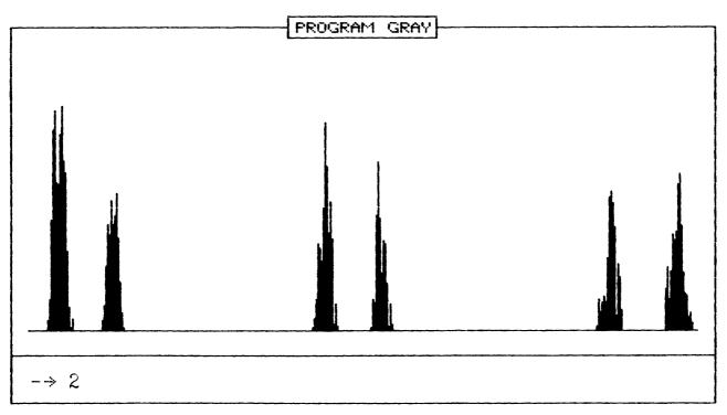
Fig.3. Normal Zeeman effect. Observation is at right angles to the field.
