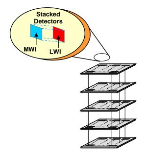
Figure 1 Vertically Integrated Sensor Architecture with multiple levels of signal processing at the detector
