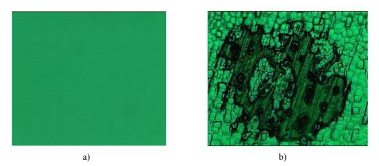
Figure 5. PECVD silicon nitride on a). standard silicon wafer and b) SiGe wafer
