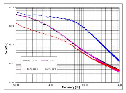
Figure 2. Low frequency noise spectrum density on the base current during a ramp temperature
