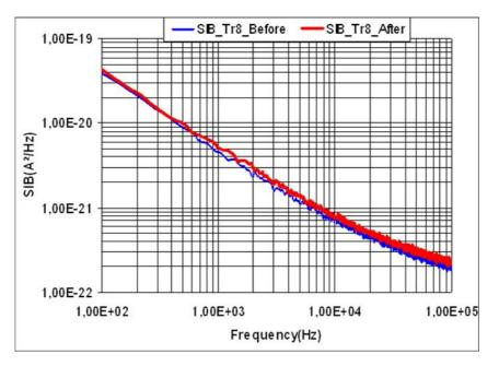
Figure 12. Low frequency noise measurement before and after post processing
