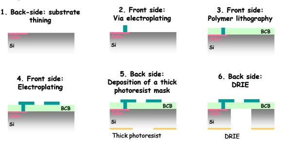
Figure 6. Micromachined above IC technological process flow
