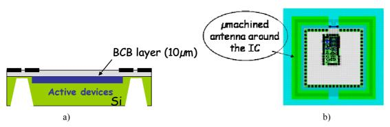
Figure 1. Schematics of an antenna with micromachined trenches: a) cross section and b) top view
