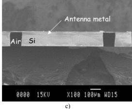
Figure 7. Pictures of an antenna with trenches seen from: a) the front side, b) the back side and c) the SEM cross section
