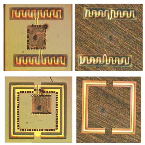
Figure 11. Examples of post-processed antennas with IC's (front and back sides)
