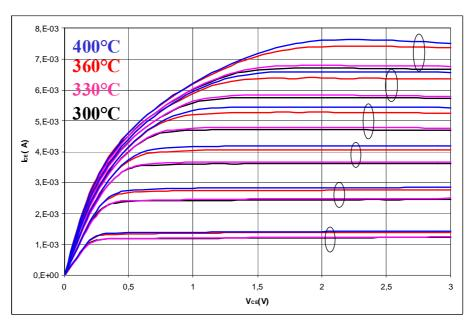
Figure 3. Static performances of a test transistor during a temperature ramp
