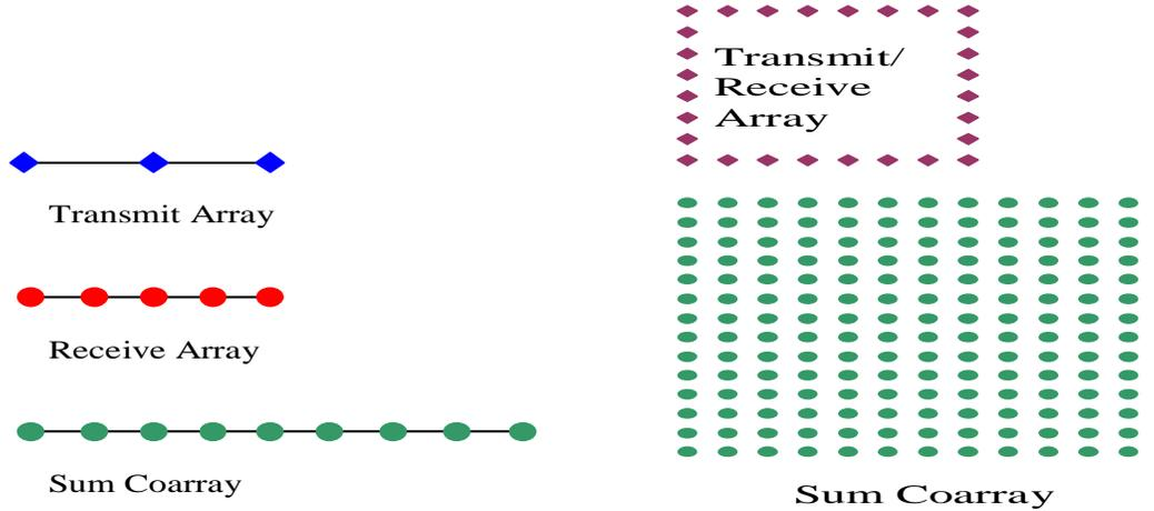
Figure 5. 1-D and 2-D Co-array examples
