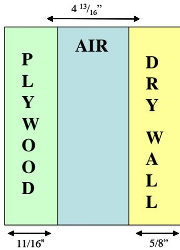
Fig. 12 Wall Characteristics
