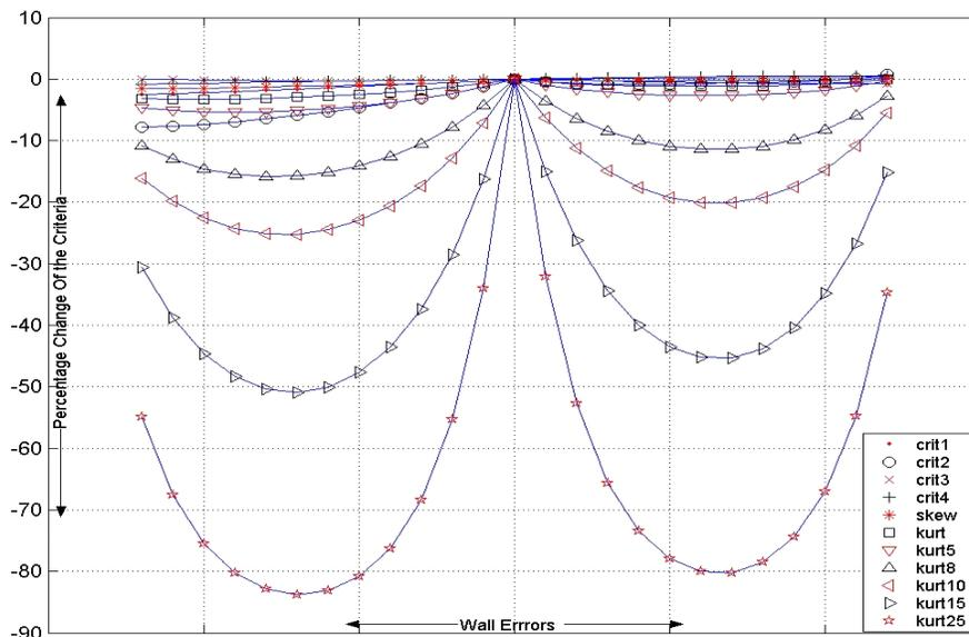
Fig 9 Percentage error change of the criteria involving just wall thickness errors in single target case
