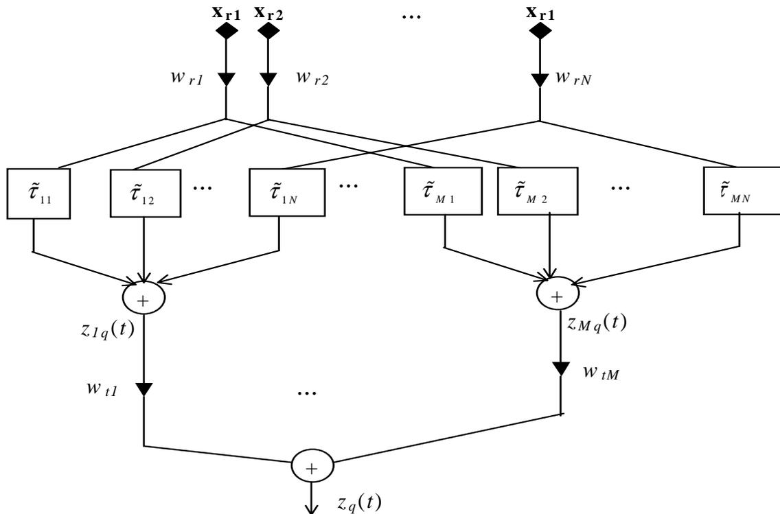
Figure 2: Block diagram of the post-data acquisition beamformer
