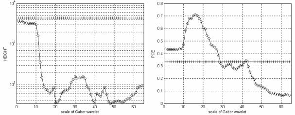
Fig.5. Gabon wavelet with various scales (height of autocorrelation peak and PCE criterion). Additionally horizontal "+" line represents value for phase only filtering (images without preprocessing step).
