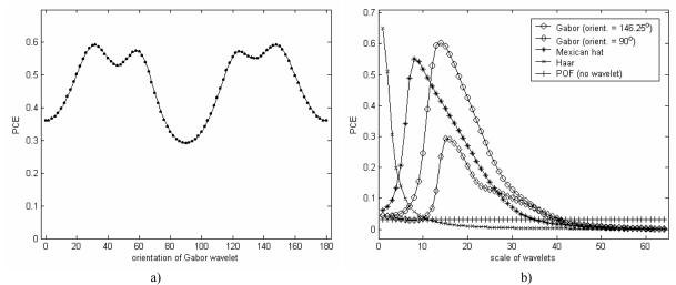
Fig. 2. Influence of wavelet parameters on the PCE value: a) influence of orientation of Gabor wavelet on PCE value, b) influence of scale of various wavelets on PCE value.
