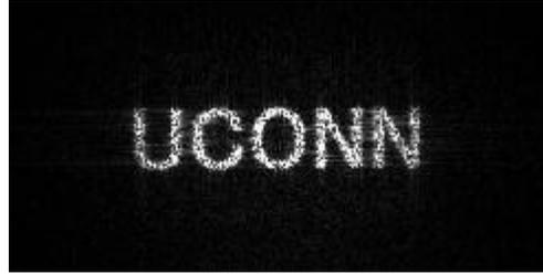
Figure 2. Image of the input object for Fresnel encryption obtained with a lensless phase-shift interferometer without reference phase mask.
