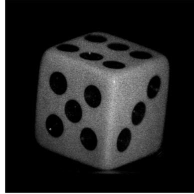
Figure 6. Image of the original 3D object to be encrypted obtained by phase-shift interferometry with the optical system in Fig. 5 without reference phase mask.
