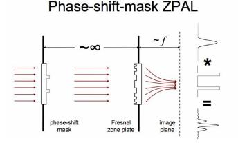
Figure 4: Schematic of a ZPAL phase-shifting strategy that would produce narrower peaks in the point-spread function, at the expense of higher sidelobes. This would be useful in exposing isolated lines or spaces but generally not for patterns of arbitrary geometry.
