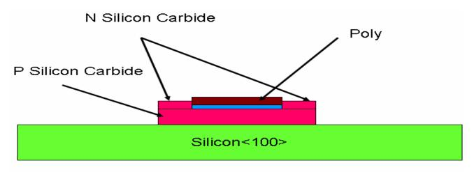
Figure 3 Schematic of single transistor memory cell
