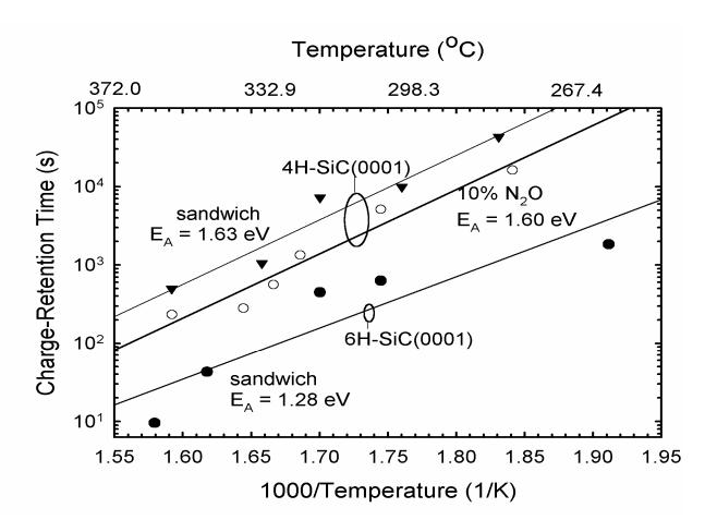
Figure 2 Retention of Non equilibrium Charge in SiC MOS Capacitors
