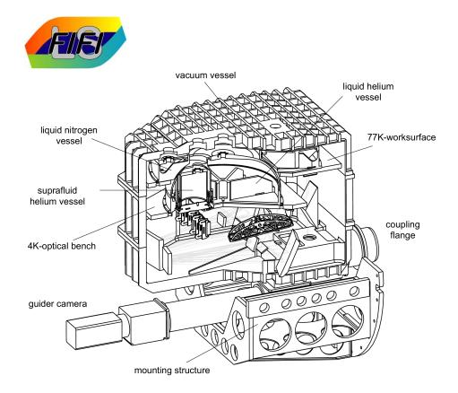
**Figure 1.** A cut through the *FIFILS* cryostat. The optical components are mounted on the work surfaces attached to the cryogen vessels. Light from the SOFIA telescope is entering the instrument from the right via the coupling flange.
