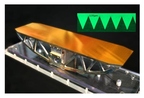
Figure 6. Gold coated "red" grating and inset with microscopic image of the grating profile (grating constant  $120 \,\mu$ m).
