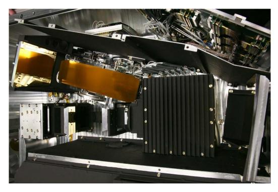
Figure 5. The "red" spectrometer: The two collimators are on the extreme right and top left. The grating on its drive assembly is next to the left collimator. Below the grating, there are the exit optics and the slices tower to the left. The black box on the right is the detector housing.
