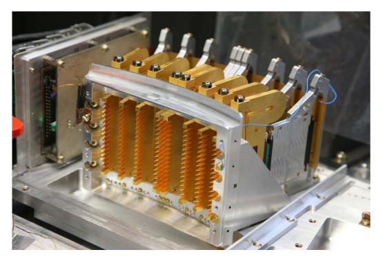
**Figure 9.** Nine detector modules in the "red" detector housing. Gold coated light cones, or light guides, are in front of the detector modules. The screw applying the stress to the column of detector pixels in the detector modules can be noticed on top of the modules. In the back, the CRE housings can be seen with spring contacts to a flexible circuit board for the electrical connection.
