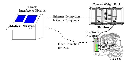
Figure 3. The three main entities in the *FIFLS* control system: the user accessible PI rack with two PCs (Maker and Master), the counter weight rack on the telescope with the control PC (Mother) and various drivers, and *FIFLS* with an electronics backpack. See Sect. 2.4 for the details.
