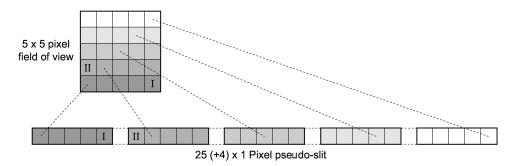
**Figure 2.** Illustration of the basic design premise for the *FIFILS* image slicer. The optics slice the rows of the  $5 \times 5$  pixel field of view into a  $25 \times 1$  pixel pseudo-slit. The pixel gaps in the slit are added to reduce cross-talk between nonadjacent field pixels (e.g. pixels I and II).
