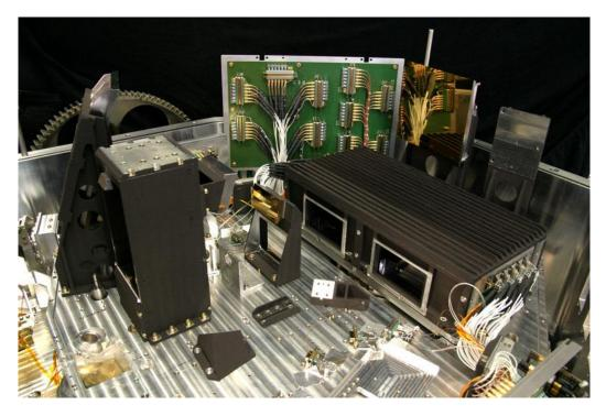
**Figure 4.** Integration in progress: The 4 K-work surface from left to right: collimator, the image slicer tower, exit optics, detector housing (on 1.9 K-work surface), collimator; in the back: pre-amplifier board with data cables.
