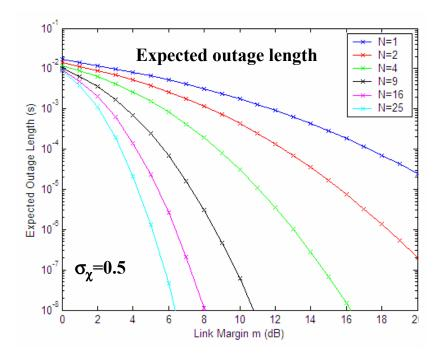
Figure 13. Expected outage length for different degrees of diversity;  $\sigma_{\chi}$ =0.5 (strong turbulence), transverse wind speed of 10 km/hr (moderate), and cutoff wind speed of 100 km/hr (nominal).
