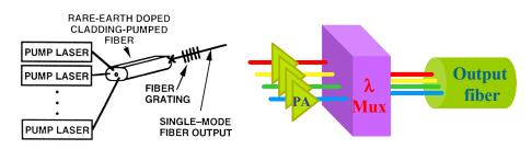
Figure 8. Double-clad erbium amplifier and multiplexer.
