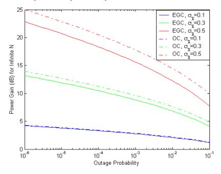
Figure 14. Power gain of direct detection diversity optical communication systems for moderate turbulence and optimum receivers (OC) and equal gain combining (EGC) receivers – infinite number of diversity receiver asymptote.
