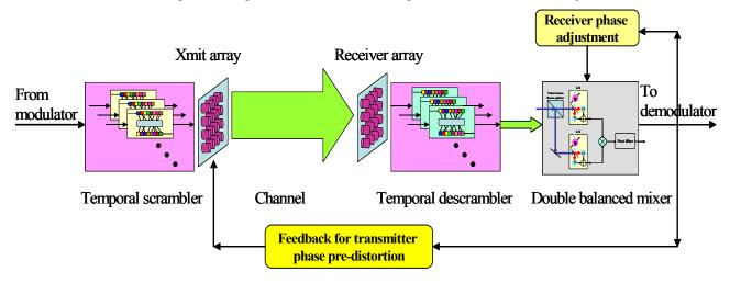
Figure 20. Transmission system block diagram; not all subsystems shown (including: modulator/demodulator, coder/decoder, frequency shifters, optical amplifiers etc.).
