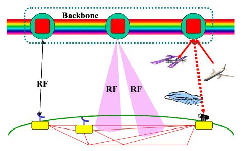
Figure 1. Integrated space-terrestrial network with intersatellite optical crosslinks and optical up and down links between satellites, ground and aircraft through clear air turbulence.
