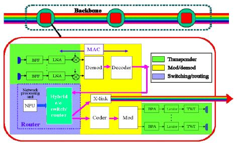
Figure 17. Different processing architecture options for a satellite network node.
