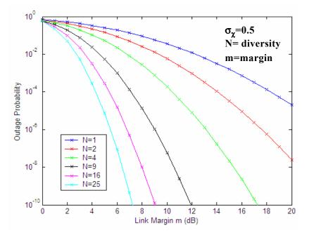
Figure 12. Outage probability for different degrees of diversity; log-amplitude standard deviation,  $\sigma_{\chi}$ =0.5 (strong turbulence), transverse wind speed of 10 km/hr (moderate), and cutoff wind speed of 100 km/hr (nominal).
