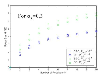
Figure 15. Power gain of direct detection diversity optical communication systems for moderate turbulence and optimum receivers (OC) and equal gain combining (EGC) receivers – finite number of receivers.
