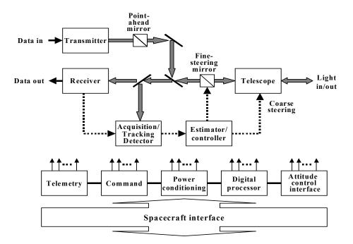
Figure 4. High-level block diagram of an optical space communication system.
