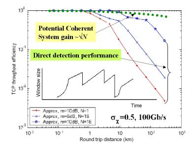
Figure 19. Transport layer throughput efficiency of incoherent and coherent 100 Gbps optical systems as a function of link distances, showing improvements due to spatial diversity and potential gains with coherent detection.
