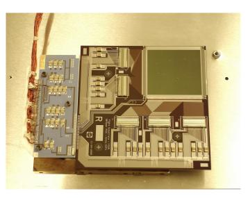
Figure 13. A quadrant of MSA system. A 171x365 MSA was bonded on a silicon substrate at the upper-right corner. The substrate was populated with addressing drive chips and all the passive components
