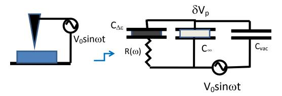
Figure 3. SPM tip above dielectric sample and equivalent circuit for noise analysis.
