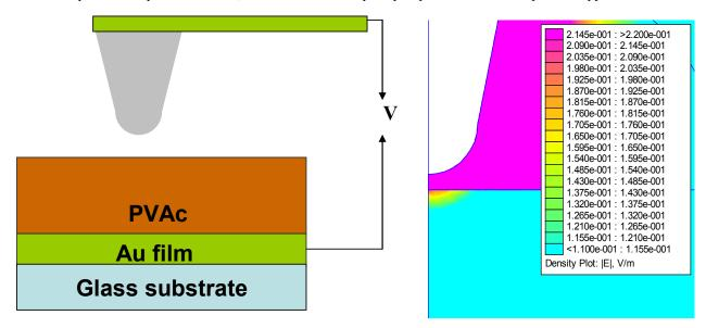
Figure 1. Measurement setup on the left, showing the conducting SPM tip and dielectric sample. On the right is a finite-element calculation, showing the electric fields dropping a factor of two in the colored region below the tip.
