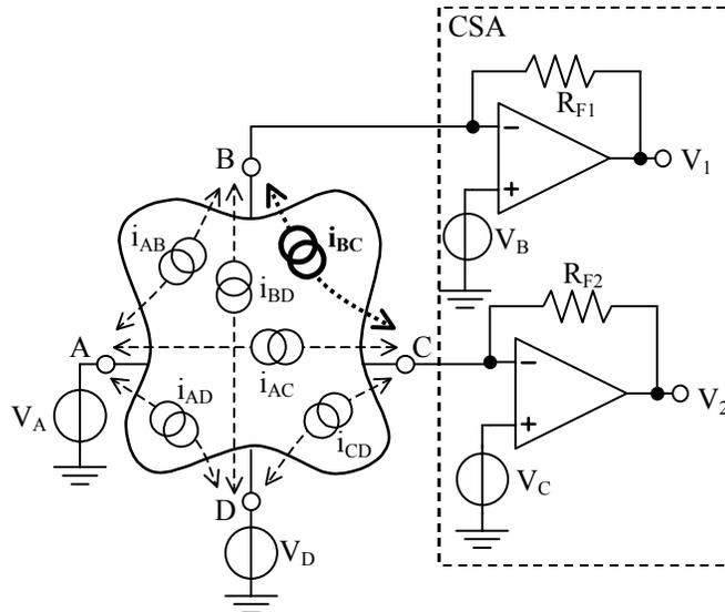
Figure 3 Schematics of the connection of the Correlation Spectrum Analyzer to a generic four-electrodes device to extract only the noise source  $i_{BC}$ .
