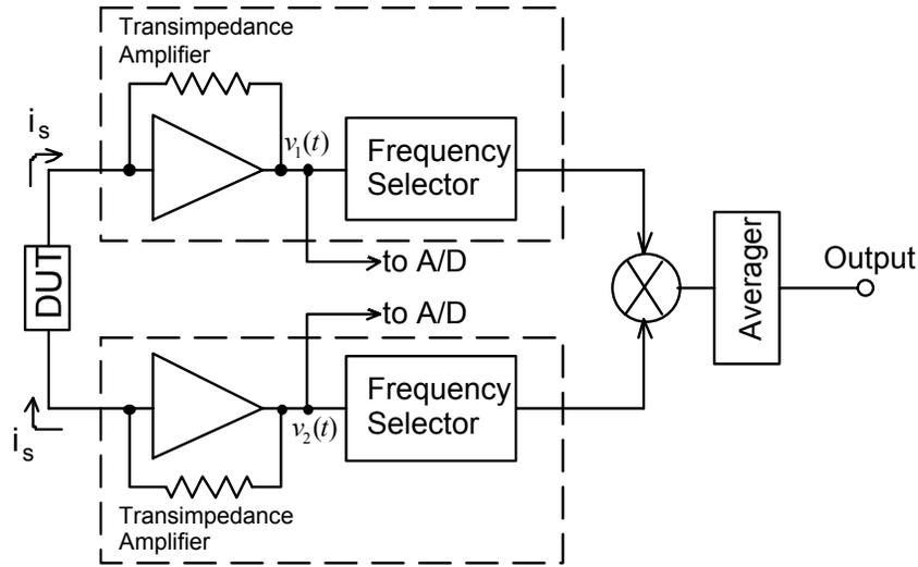
Fig. 1. Scheme of a Correlation Spectrum Analyzer.
