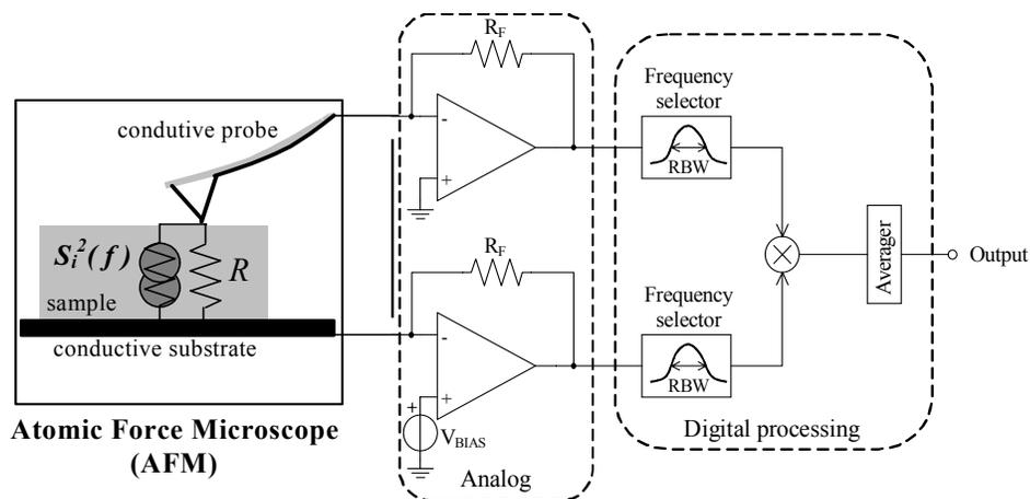
Figure 5 Diagram of the experimental set-up for nanoscale noise spectroscopy. The atomic force microscope (AFM) is connected to two wide-bandwidth current-to-voltage amplifiers in a correlation spectrum analyzer scheme to perform high sensitivity noise spectroscopy measurement.
