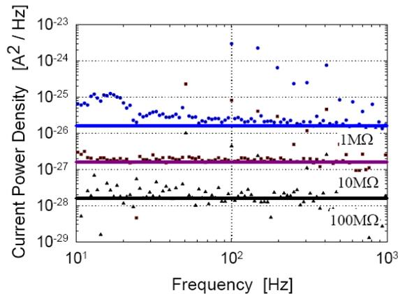
Fig. 6. Noise spectroscopy using AFM of discrete resistor of well-known value ( $1\text{M}\Omega$ ,  $10\text{M}\Omega$ ,  $100\text{M}\Omega$ ) connected in series of a gold substrate. Solid lines indicate the corresponding theoretical level of Nyquist noise, showing excellent agreement with measured data.
