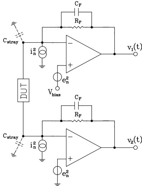
Figure 2. Schematics of instrument input stage for the case of a current sensitive set-up. Main noise sources, parasitic capacitances and DUT impedance are indicated to help in the evaluation of the spurious correlated signal that set a lower limit in the instrument sensitivity.
