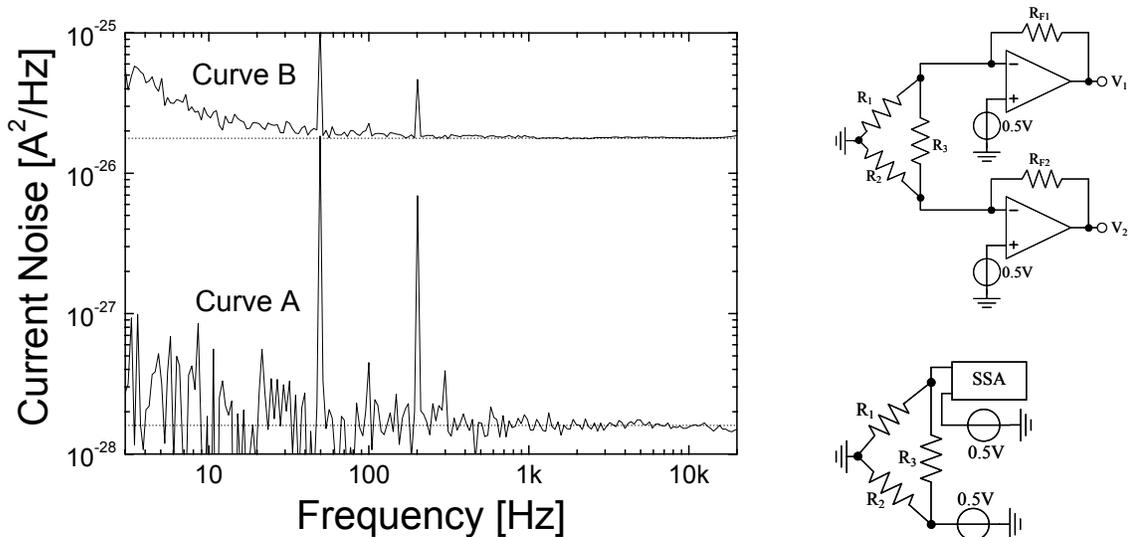
Figure 4 Current noise spectra obtained from the resistive network connected as in the configuration at the right top or connected to a single channel spectrum analyzer (SSA) as in the configuration at the right bottom. The noise produced by  $R_3$  can only be sorted out by using CSA after a measuring time of  $T_m \approx 4$  hours.
