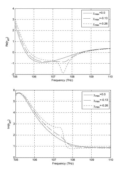
Fig. 3. Real [upper] and imaginary [lower] parts of the refractive index of nano-dispersed dye-doped nematic liquid crystals showng enhanced negative index behavior and a lowered loss [smaller imaginary refractive index]
