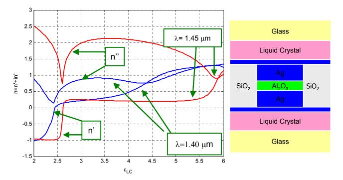
Fig. 4. Plots of real [n' - lower two curves] and imaginary [n" - upper two curves] parts of the complex refractive index of the liquid crystal clad metallo-dielectric nano-structures for various values of the liquid crystal dielectric constant and two laser wavelengths.
