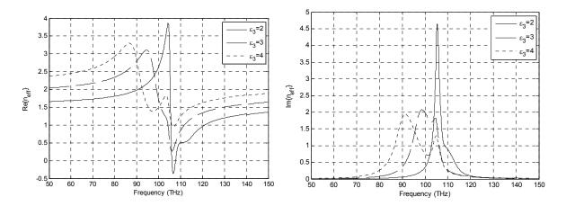
Fig. 2 Real [left] and Imaginary [right] parts of the complex effective refractive index of the core-shell nano-spheres dispersed nematic liquid crystals showing tunable refractive index from negative to positive values.
