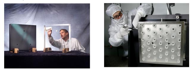
Fig. 4 Example of an unsolarized and solarized transport mirror (left image). NIF deformable mirror undergoing wavefront validation testing (right image).
