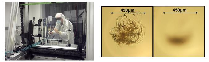
Fig. 5 NIF multilayer transport mirror being inspected after laser conditioning (left image). Crack elimination in a fused silica initiation site which has been mitigated by a doubled CO<sub>2</sub> laser (right image).
