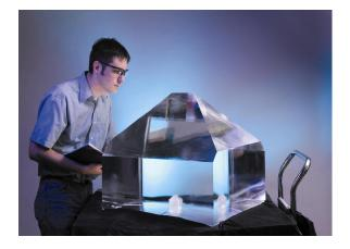
Fig 2. KDP doubler crystal grown using the rapid growth technique (left image). Final assembly of the PEPC utilizing KDP to rotate the beam polarization as part of an optical switch (right image).
