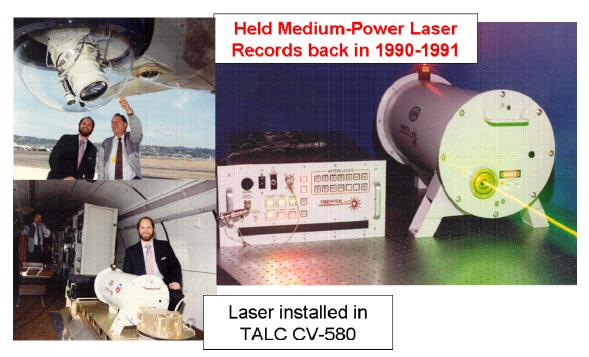
0.5J @ 20 Hz, 532 nm center wavelength, and ~2.5% wallplug efficiency
