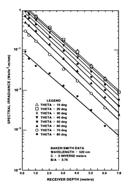
Figure 5, Comparison of  $F_w(\Theta)$  and Experimental Data
