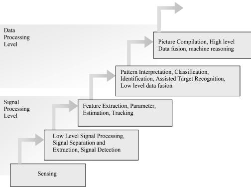
Figure 1: Signal and Data Processing Chain
