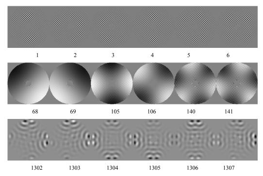
Figure 4: SAXO eigen modes, ordered by increasing eigen values (mode number below). The first ones (top) are related to waffle modes, the last (bottom) to Fourier modes. But among the first eigen modes (middle) also exists highly energetic turbulent modes (very close to coma, astigmatism ...).
