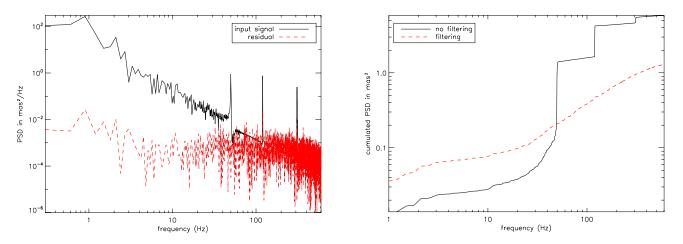
Figure 7: left, input and residual PSD of the  $S_2$  mode on which the vibrations are introduced with vibration filtering. Right: cumulated PSD of residual  $S_2$ , mode with or without filtering.
