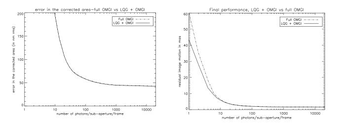
Figure 8: left SAXO final performance in residual error (in nm rms) according to flux. Right: SAXO final performance in residual image motion (in mas rms) according to flux.
