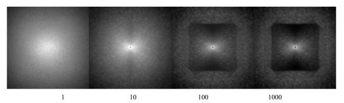
Figure 9: Coronagraphic PSFs for various flux in photons/sub aperture/frame.
