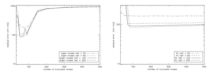
Figure 6: Impact of basis truncation respectively for the eigen mode basis (left) or the KL basis (right) for various flux (20, 60, 120 and 200 photons/frame/sub-aperture) in terms of overall residual error (nm rms).
