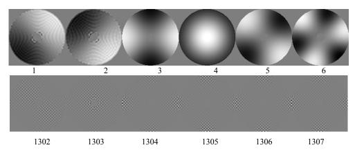
Figure 5: SAXO KL modes, ordered by increasing mode number, which is also by decreasing turbulent energy.
