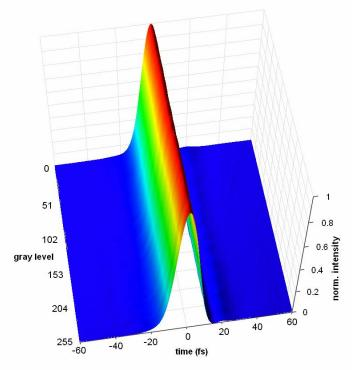
Fig. 5. High-fidelity temporal transfer function of a PAN type LCoS-SLM represented by the pulse profile as a function of the gray value. The pulse shape was measured with LX-SPIDER technique<sup>46</sup>.
