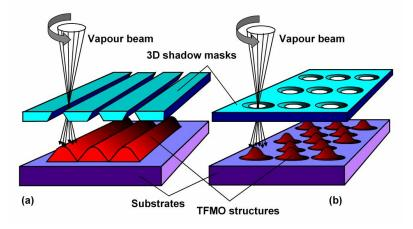
Fig. 2. Deposition of arrays of TFMO with multiple miniaturized shadow masks consisting of (a) slit-array masks, (b) hole masks enabling for the bottom-up fabrication of linear and 2D arrangements of cylindrical and circular, micro- or nanoscale single (layer or multilayer) structures, respectively (schematically, after<sup>1</sup>).
