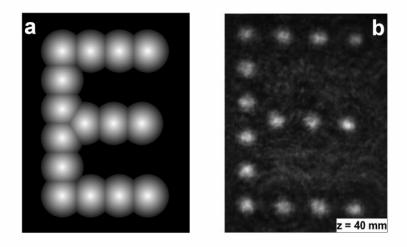
Fig. 7. Nondiffracting image generated with adaptive liquid-crystal microoptics: (a) programmed gray value map (horizontal period 387  $\mu$ m), and (b) propagated distribution ("flying image") detected at a distance of z = 40 mm behind the LCoS-SLM (laser pulse duration < 20 fs). In the left picture, all substructures act as separately addressable reflective axicons of variable conical angle.
