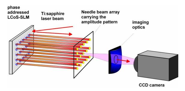
Fig. 6. Programmable needle beam arrays for the generation of "flying images". An image information is written in the spatial light distribution by addressing individual phase elements of an LCoS-SLM. The plane of interest is imaged onto a CCD-camera (schematically).
