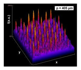
Fig. 4. Spatial intensity distribution of a hexagonal array of 10-fs needle-shaped nondiffracting beams generated with ultraflat reflective static TFMO axicons (angle of incidence  $> 25^{\circ}$ ).
