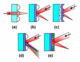
Fig. 3. Different types of TFMO structures: (a) refractive (dielectric), (b) pseudo-reflective (dielectric on metal), (c) reflective (metal on dielectric), (d), refractive-diffractive (dielectric on grating), and (e) adaptive pseudo-reflective structure (liquid-crystal layer on metal mirror with glass cover plate and segmented electrodes).
