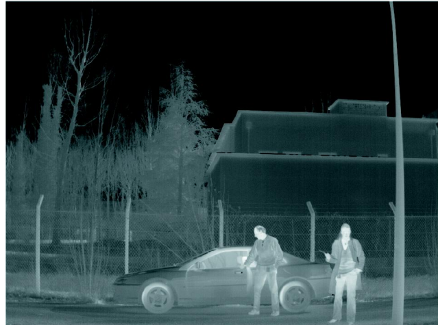
Fig. 26. Image taken with a 1024 \times 768 \alpha -Si microbolometer with 17 \mu\text{m} pixels as described in paper -62.
