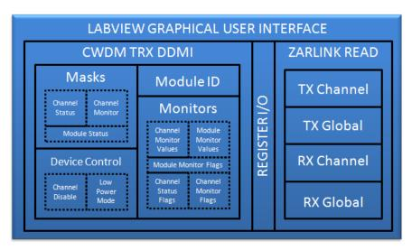
Fig. 7. LabView user interface architecture used for module development.
