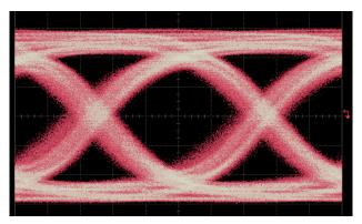
Fig. 4. Eye diagram of 10Gbps operation of an OptiComp Corp. prototype WDM transceiver module.
