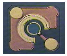
Fig. 3. PIN photodiode fabricated at OptiComp Corp. that can be bonded to an optical bench for a vertical submount in the receiver module.
