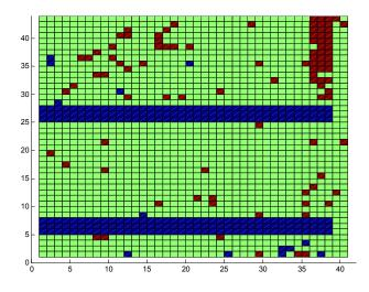
Fig. 2. Fabrication of VCSELs is a high yield process with nearly 95% passing all wafer-level LIV conformance, shown in green, versus those not passing (shown in red).
