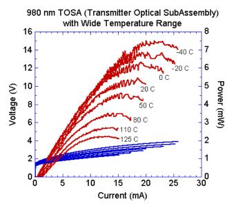
Fig. 7. Excellent operational characteristics of VCSELs over a wide temperature range eliminates the need for active cooling of the transceiver module.
