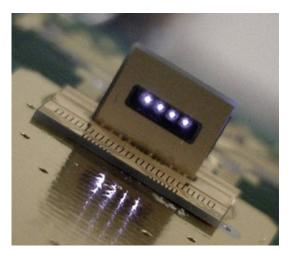
Fig. 6. Prototype transmitter sub-assembly with four VCSELs mounted on vertical submount.
