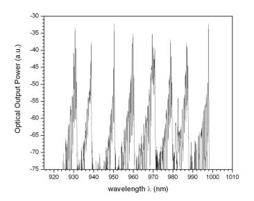
Fig.8. Channel outputs of VCSELs mounted on optical benches as observed in a prototype transceiver module.
