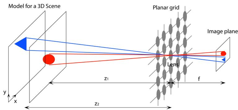
Fig. 1. Pickup process in integral imaging (II) having a synthetic aperture.
