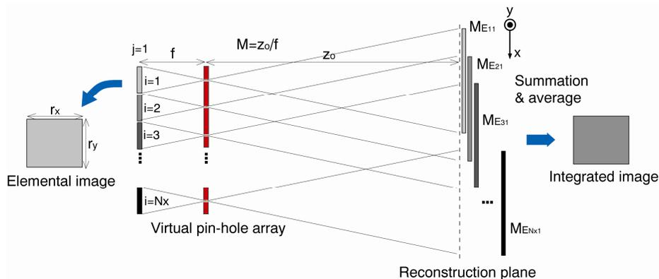
Fig. 2. Computational reconstruction in integral imaging (II).
