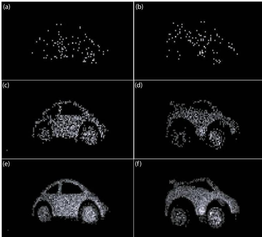
Fig. 6. Sectional images of the 3D scenes reconstructed from very small number of photons-counted elemental images, where the  $10 \times 10$  elemental images set was generated with the photon counting detection model.  $\tilde{N}$  is the expected number of photons per elemental image. (a) Car I with  $\tilde{N} = 1$ , (b) Car II with  $\tilde{N} = 1$ , (c) Car I with  $\tilde{N} = 11$ , (d) Car II with  $\tilde{N} = 11$ , (e) Car I with  $\tilde{N} = 51$ , (f) Car II with  $\tilde{N} = 51$ .
