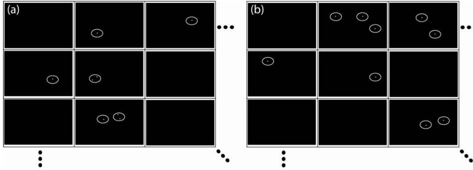
Fig. 5. Subset of elemental images having small number of photons generated according to a photon counting detection model. (a) car I and (b) car II.
