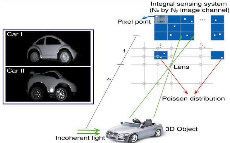
Fig. 3. Schematic setup of II system with camera array for 3D object visualization and recognition.
