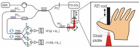
Figure 1: Schematic of the fibre-based OCT system employing balanced optical quadrature detection and the experimental geometry.
