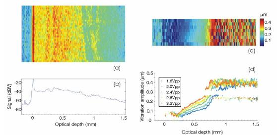
Figure 2: OCT A-scan and OCE-derived vibration amplitude versus optical depth for human skin *in vivo*: (a) OCT image without applied vibration; (b) Average A-scan; (c) Vibration amplitude image for PZT drive voltage of 2.4Vpp; and (d) Average vibration amplitude for various PZT drive voltages.
