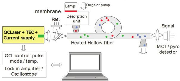
Fig. 37 Set up using quantum cascade laser for the detection of explosive materials as described in paper -137.
