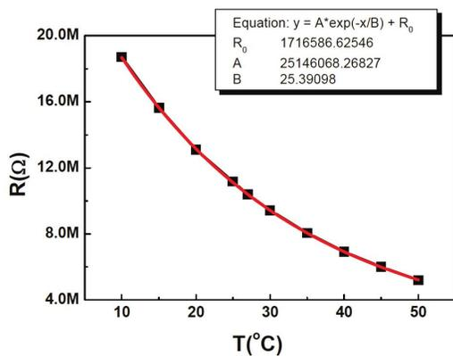
Fig. 7 Temperature dependence of a nickel-oxide film with a TCR of 3.3 % at 27 °C from paper -142.
