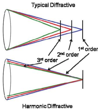
Fig. 9 Paper -36 shows improved color correction with harmonic diffractive design.
