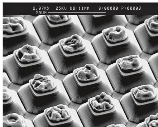
Fig. 18 Dry-etched pixels of MOVPE-grown HgCdTe on GaAs substrates reported in paper -74.
