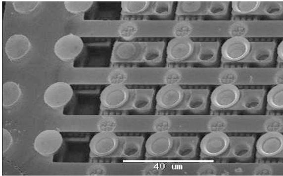
Fig. 5 Dual band QWIP array details. The pixels are on a 25 μm pitch—from paper -15.
