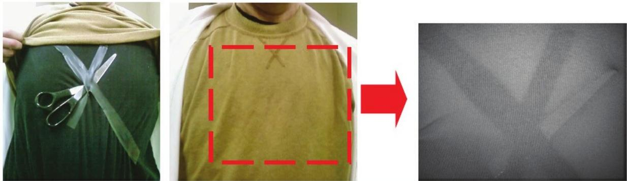
Fig. 36 Illustration of near-infrared detection of concealed objects under clothing—from paper -157.
