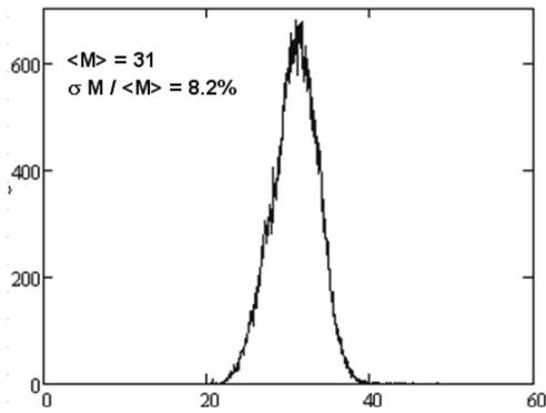
Fig. 28 Histogram of APD gain at 6 V reverse bias as described in paper -106.
