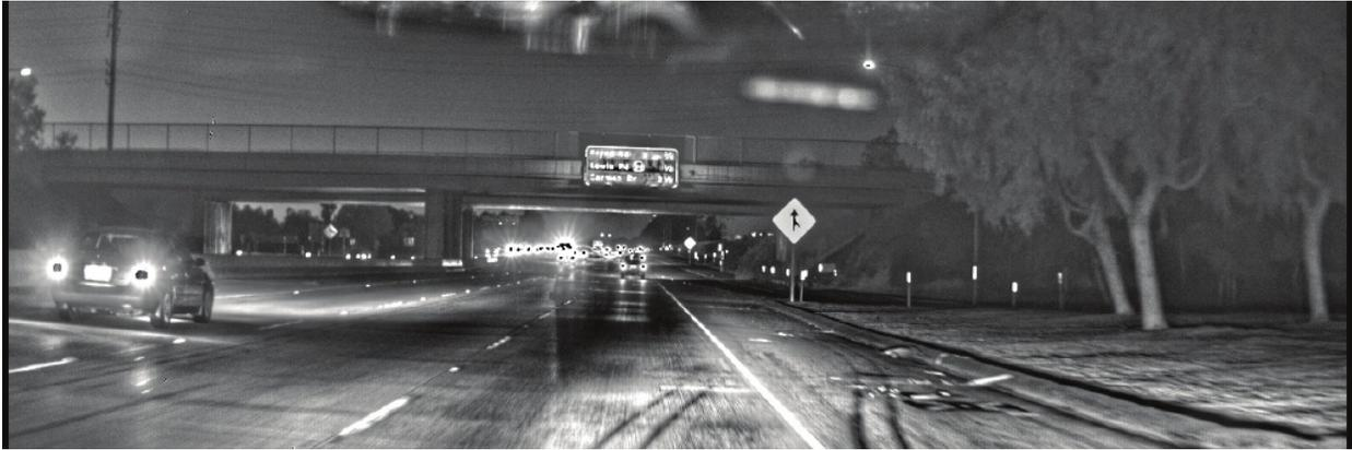
Fig. 31 SWIR image from paper -116 using a MANTIS III camera and local-area contrast to bring out detail from dark areas and suppress saturation in bright areas.
