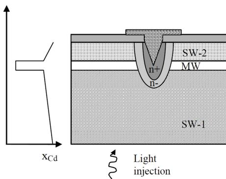
Fig. 29 Horizontal gain well APD structure from paper -107.
