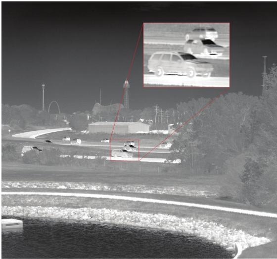
Fig. 3 Corrugated QWIP imagery from a  $1024 \times 1024$  format array described in paper -07.
