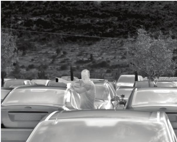
Fig. 32 From paper -124 showing imaging from a  $1280 \times 1024$  InSb FPA with  $15 \mu\text{m}$  pixels.
