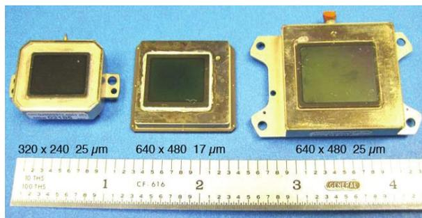
Fig. 8 Comparison of VO<sub>x</sub> microbolometer packages from paper -27.
