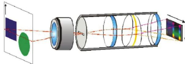
Fig. 33 Hyperspectral imaging spectrograph in which a line on the image is dispersed via a prism-grating-prism optical assembly and recorded by a SWIR camera—from paper -127.
