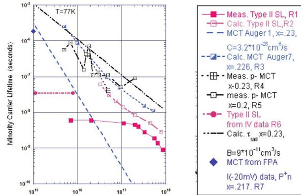
Fig. 16 Measured and calculated minority carrier lifetime for LWIR p- and n-type MCT and p-type LWIR Type II InAs/GaSb superlattice materials. Details are in paper -67.
