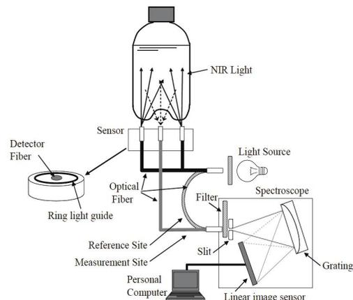
Fig. 38 Bottle inspection system for airport liquid inspection as reported in paper -145.
