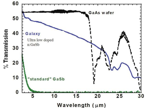
Fig. 34 Ultra-low-doped GaSb substrate material shows much higher transmission than standard GaSb—from paper -136.
