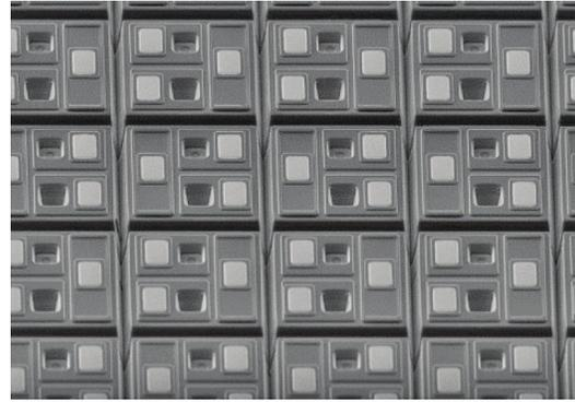
Fig. 15 A portion of the  $384 \times 288$  two-color MW/MW Type II SLS detector array in paper -64.
