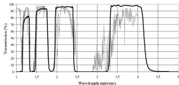
Fig. 26 Transmission of a filter (dark line) designed to transmit the atmospheric windows as described in paper-88.
