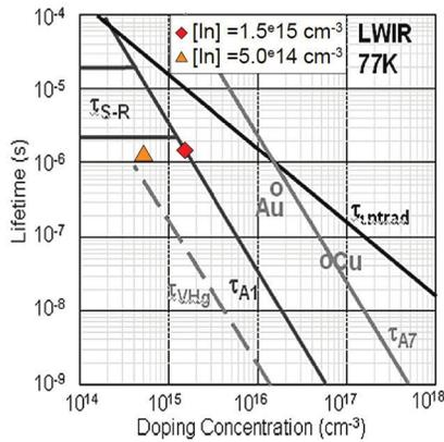
Fig. 20 Minority carrier lifetime exceeds 1  $\mu$ sec for two indium-doped LWIR samples at 77 K discussed in paper -77.
