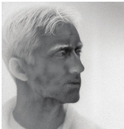
Fig. 2 MWIR InGaSb-InAs Type II MWIR superlattice FPA image in a  $1024^2$  format having  $19 \mu\text{m}$  pixels from the JPL/Raytheon paper -04.
