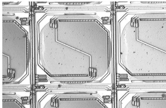
Fig. 6 Details of an 80 × 60 uncooled thermopile array from paper -23.
