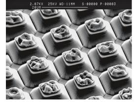
Fig. 18 Dry-etched pixels of MOVPE-grown HgCdTe on GaAs substrates reported in paper -74.
