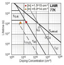
Fig. 20 Minority carrier lifetime exceeds 1 µsec for two indium-doped LWIR samples at 77 K discussed in paper -77.
