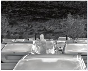
Fig. 32 From paper -124 showing imaging from a  $1280 \times 1024$  InSb FPA with 15 µm pixels.
