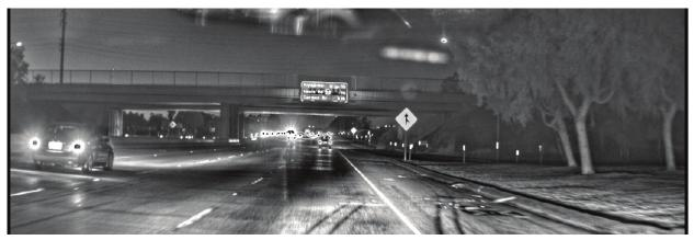
Fig. 31 SWIR image from paper -116 using a MANTIS III camera and local-area contrast to bring out detail from dark areas and suppress saturation in bright areas.
