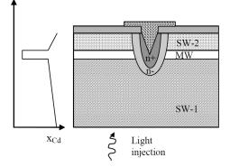
Fig. 29 Horizontal gain well APD structure from paper -107.
