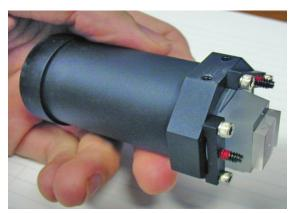
Fig. 1 A compact Dyson spectrometer from JPL paper -03.
