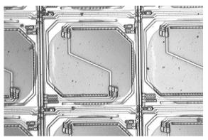
Fig. 6 Details of an  $80 \times 60$  uncooled thermopile array from paper -23.
