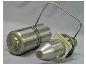
Fig. 4 Integrated  $256 \times 256$  LWIR QDIP detector-cooler assembly described in paper -13.
