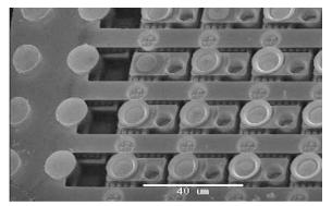
Fig. 5 Dual band QWIP array details. The pixels are on a 25 µm pitch—from paper -15.
