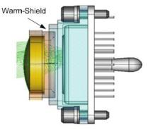
Fig. 24 Detector warm shield described in paper -135
