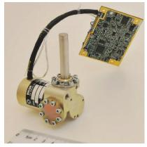
Fig. 11 Microminiature cryocooler with digital controller, from paper -45.
