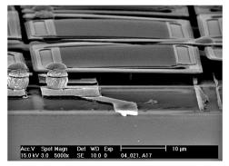
Fig. 25 Uncooled microbolometer pixel from paper -149.
