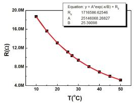
Fig. 7 Temperature dependence of a nickel-oxide film with a TCR of 3.3 % at  $27 \degree$ C from paper -142.
