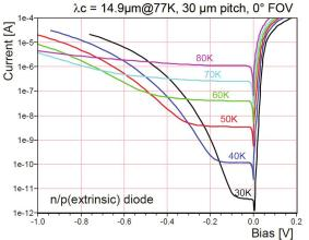
Fig. 19 Diode leakage current for an n-on-p implanted diode described in paper -75.
