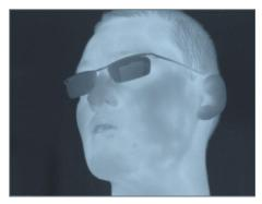
Fig. 23 Image from TEC-less  $320 \times 240$  microbolometer presented in paper-84.
