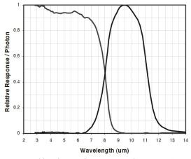
Fig. 17 Dual-band LWIR/LWIR spectral response from and MBE-grown HgCdTe array described in paper -72.
