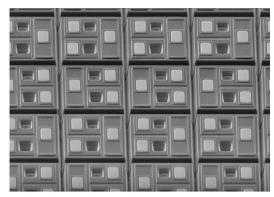
Fig. 15 A portion of the 384 × 288 two-color MW/MW Type II SLS detector array in paper -64.
