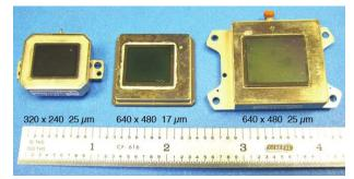
Fig. 8 Comparison of VOx microbolometer packages from paper -27.
