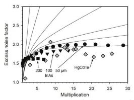
Fig. 30 Excess noise factor for InAs APDs compared with HgCdTe APDs reported in paper -112.
