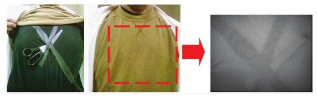
Fig. 36 Illustration of near-infrared detection of concealed objects under clothing-from paper -157.
