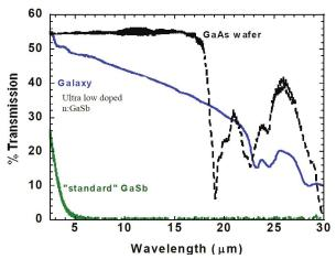
Fig. 34 Ultra-low-doped GaSb substrate material shows much higher transmission than standard GaSb —from paper -136.
