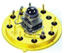
Fig. 21. Optically-immersed, LWIR HgCdTe detector described in paper -159. The lens is formed from the GaAs detector substrate.
