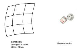
Figure 5. Spherically arranged electro-holographic display design
