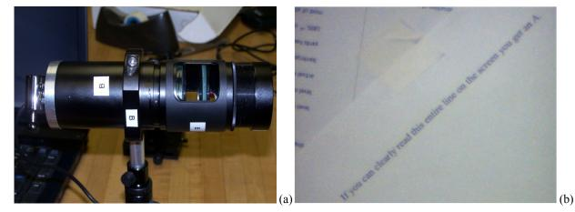
Figure 3. Image of the (a) student designed lens prototype and (b) target line captured by the webcam.
