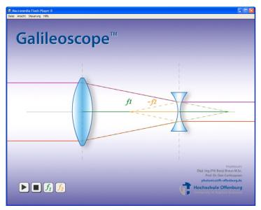
Figure 16a: Galileoscope $^{TM}$ , optical path
