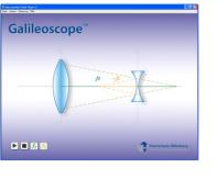
Figure 16b: Galileoscope<sup>TM</sup>, lens geometry
